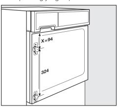
2 Mark the two hinge holes and the four smaller holes as shown in the diagram.
